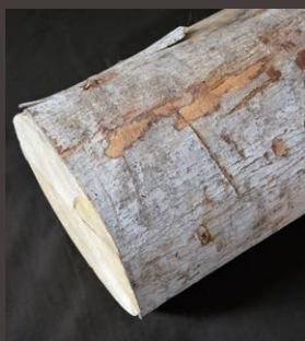
ほぼ全ての製品の原材料となるファルカタ原木 Falcata lumber is used as the raw material for almost all products.
